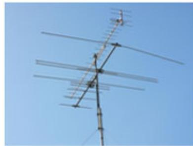
Poorly constructed antenna with inadequate antenna spacing
